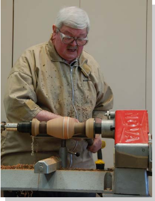
Shown here is Jim turning the exterior shape of both the top and bottom halves of the vessel.
