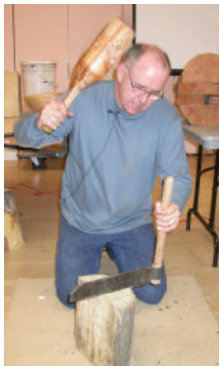
Don’t mess with Wayne and his froe! Here he shows how to split a log along the grain for spindle stock.
