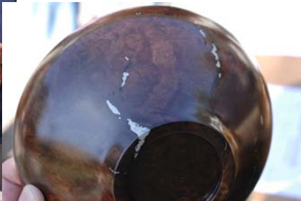
Left & Below: Dave Plemons used solder for the inlay material on this walnut bowl..Biggest problem is to get the solder to stick to the wood.
