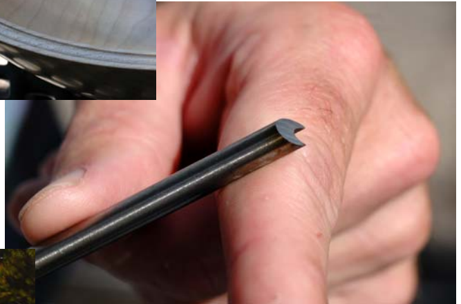
Below & Left: Brad Adams has a new beading tool made from a 1/4 inch spindle gouge.
