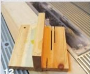
12 Make a simple jig for holding the taper while cutting the slots in the tone chamber.
