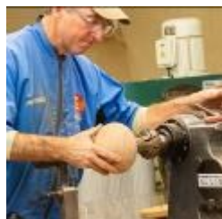
Checking fit of threads
