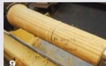
9 Turn the handle area to a cylinder but do not remove the pencil lines.
