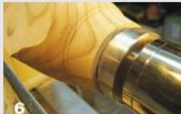
6 Begin at the tailstock end and turn the walls to about 1/8" (3mm) thick.
