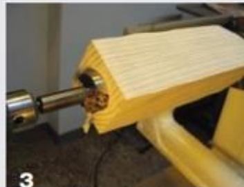
3 Using a 1½" (40mm) Forstner bit chucked in the tailstock, drill a hole 3"-4" (80mm-100mm) deep.
