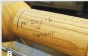
8 Measure the depth of the chamber to determine where to begin turning the handle.
