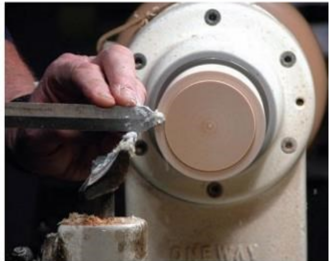
With the handle held too high, the wood is being scraped, not cut, with the tool.
