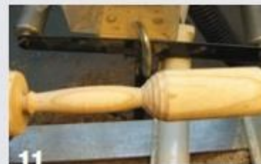
11 Form the handle and sand the tapper.
